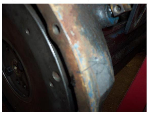
Then using a 7/8" hole saw I drilled a larger window hole after removing the fly wheel. Again I measured the circumference of the fly wheel where the marks should go and divided that by 360 to get the distance of 1° of the fly wheel and multiplied that to get the measurements for the timing marks using the small mark I drilled on the fly wheel.
