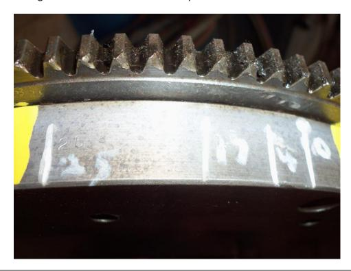
After I have reinstalled the fly wheel I will use a small bolt with a point ground on the end and drill and tap a hole through the block where it bolts to the transmission aimed at the TDC timing mark. This is what I ended up with after adding side distributer type timing marks on my front mount distributer 9N engine block.
