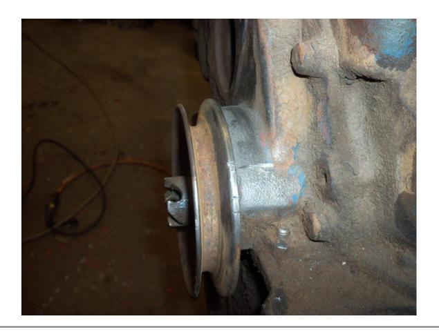
I made a pattern off of my 50 8N where the timing window is. To install timing marks on the fly wheel. Using I drilled a small hole through the block and put a small mark on the fly wheel.
